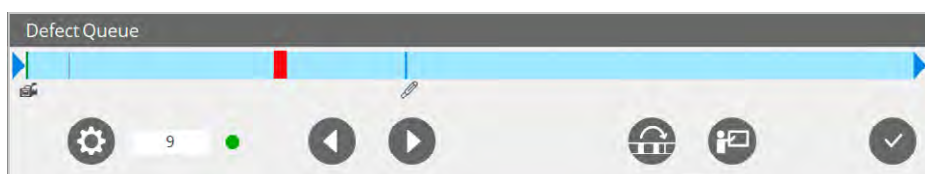
Placement control allows pinpoint positioning of a selected defect on the doctor machine.
