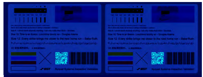
The UV illumination makes the QR code clearly visible for inspection
