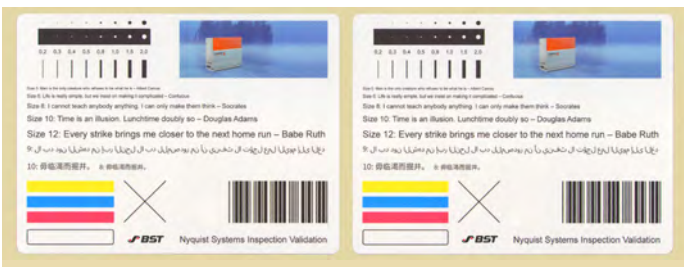
Standard illumination: The QR code printed with transparent luminescent ink is invisible
