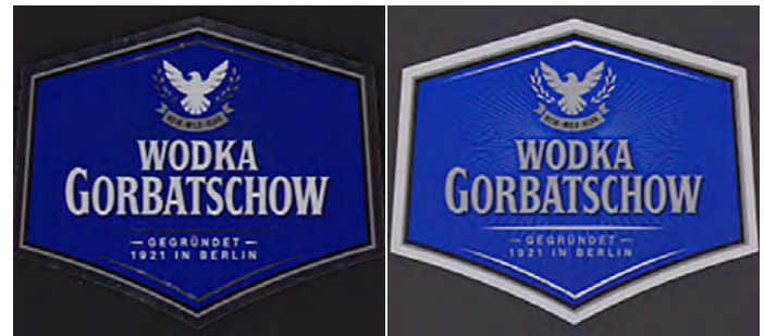
Camera image with dark field illumination
